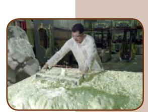
The entire under area of the spa shell is 70% foam filled with high-density structural foam for additional insulation and support. This allows for maximum support and insulation, while enabling access to over 90% of plumbing in case a repair is necessary in the future life of the spa.
